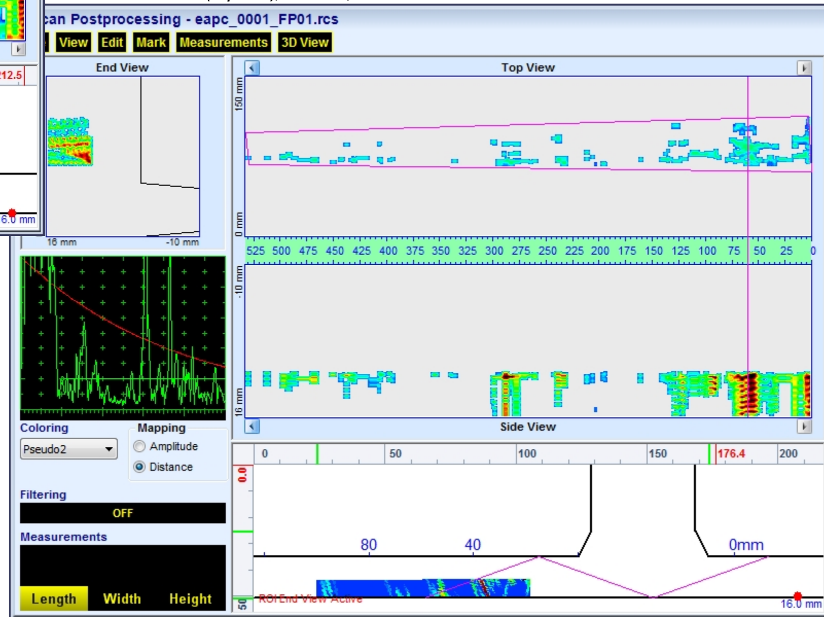
C-Scan (Top View), Side View, End View Data for the scattered corrosion inside the tank at the soil side
