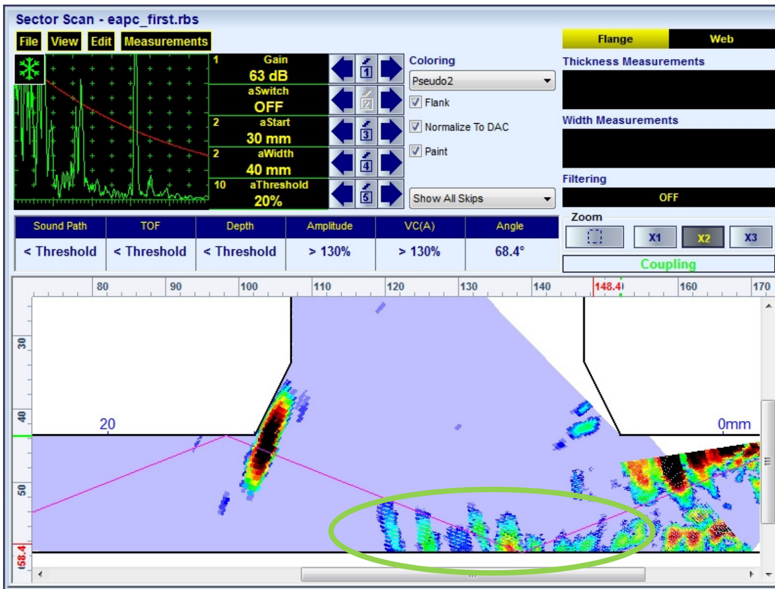
True-to-Geometry Sectorial Scan Coverage
