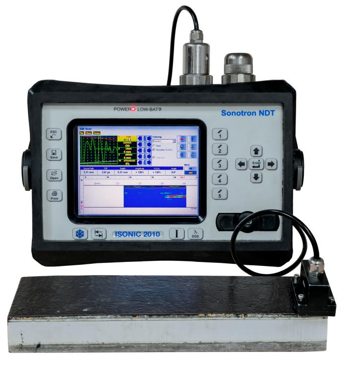
Compression wave 0-deg B-Scan coverage combined with nonlinear acoustics approach allowed by the powerful PA pulser receiver of ISONIC 2010 ensures detection of the imperfections over entire volume of the extremely attenuating glass-fiber-(GFRP) and other heavy composite-made parts with use of the same high frequency highly damped PA probes, which are well suitable for the regular metals inspection
