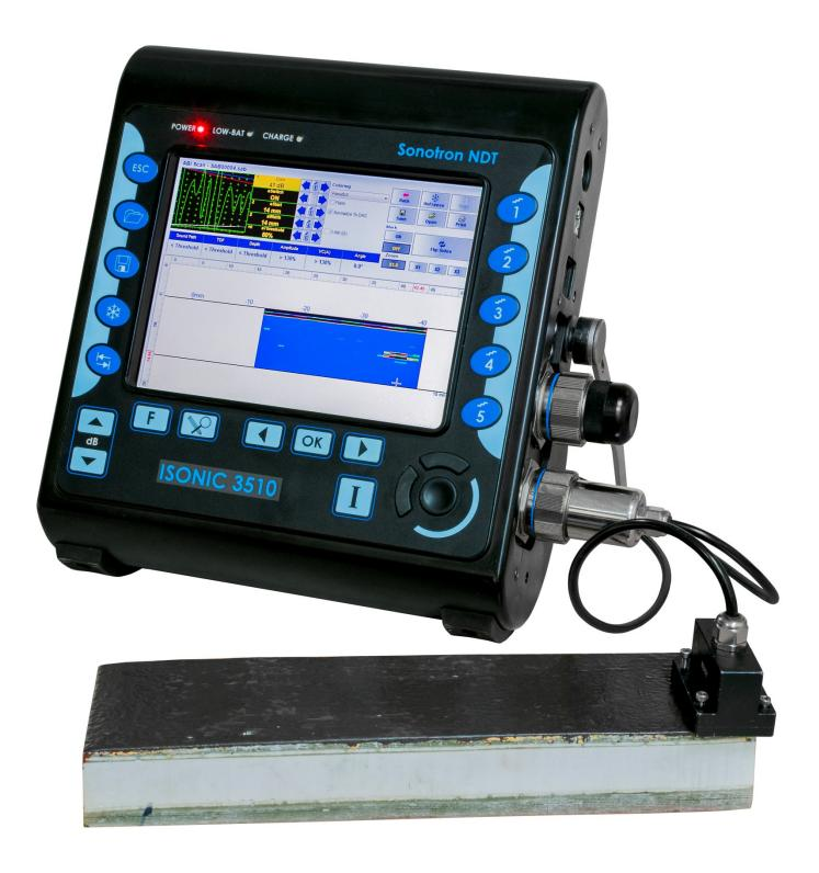
Compression wave 0-deg B-Scan coverage combined with non-linear acoustics approach allowed by the powerful PA pulser receiver of ISONIC 3510 ensures detection of the imperfections over entire volume of the extremely attenuating glass-fiber-(GFRP) and other heavy composite-made parts with use of the same high frequency highly damped PA probes, which are well suitable for the regular metals inspection
