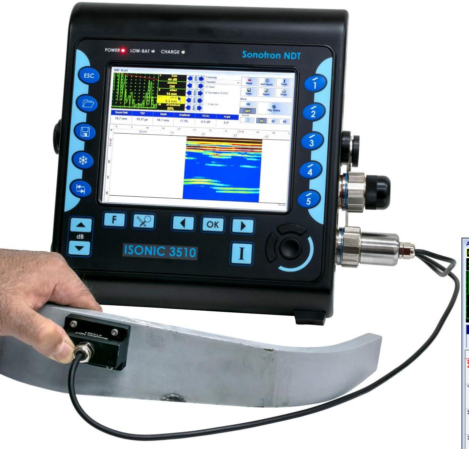
Compression wave 0-deg B-Scan coverage combined with nonlinear acoustics approach allowed by the powerful PA pulser receiver of ISONIC 3510 ensures detection of the imperfections over entire volume of the extremely attenuating glass-fiber-(GFRP) and other heavy composite-made parts with use of the same high frequency highly damped PA probes, which are well suitable for the regular metals inspection
