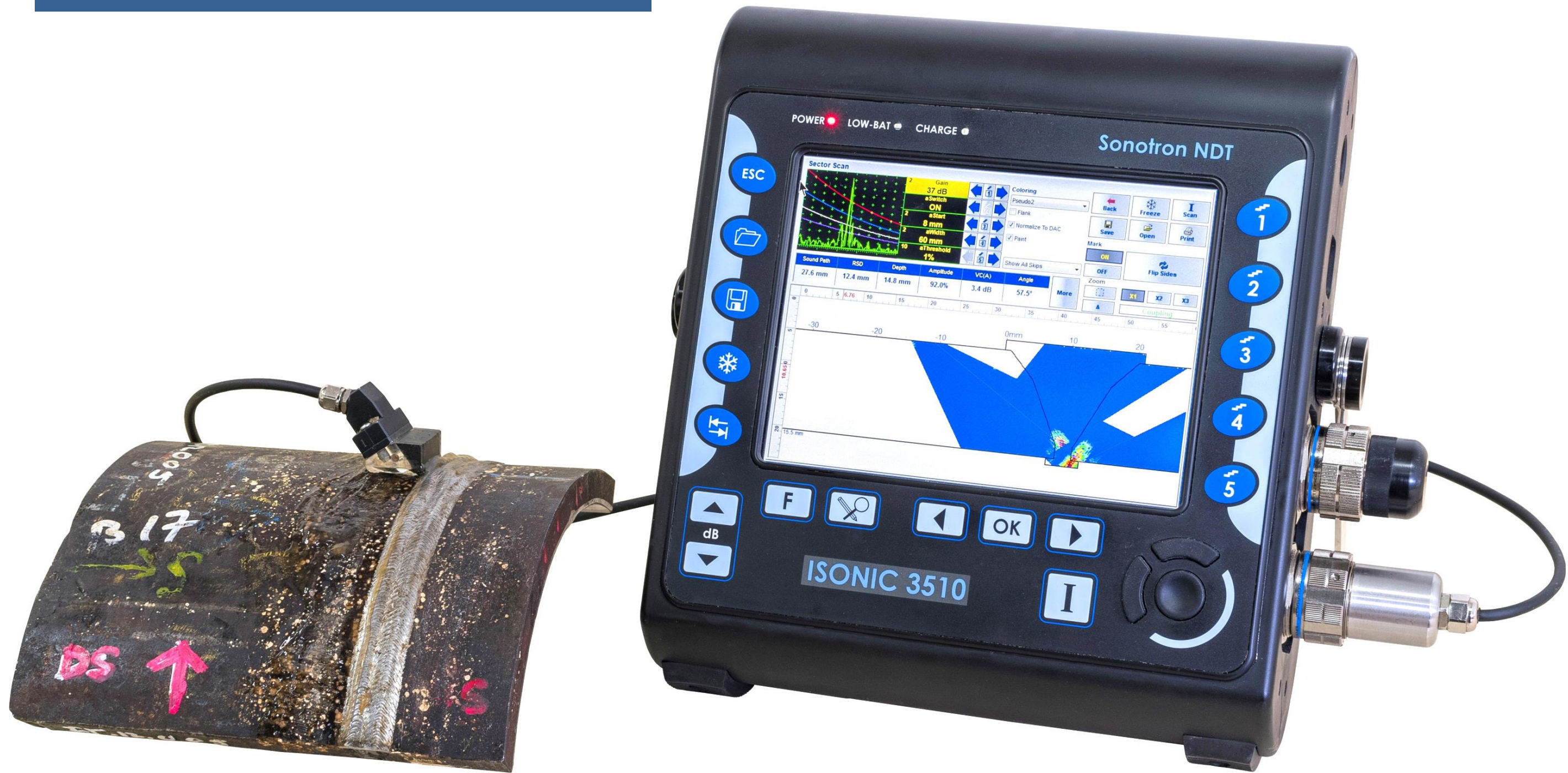
CRA Butt Weld (Hastelloy C-276) in the Cladded Pipe: TTGI C-Scan
