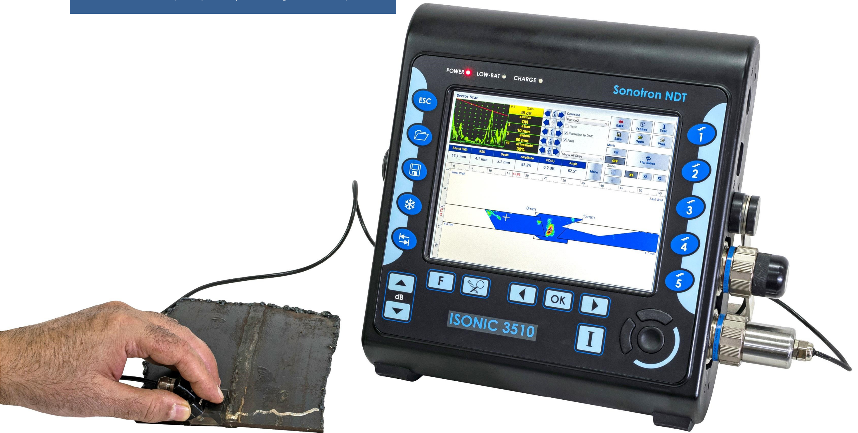
Spiral Weld: TTGI S-Scan
