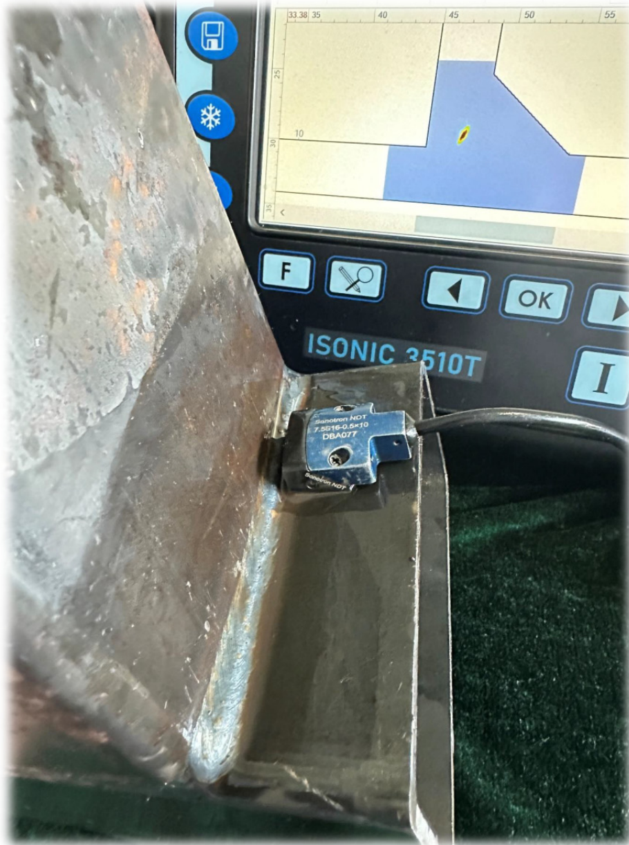
Structural straight corner weld between thin wall hollow rectangle profiles
