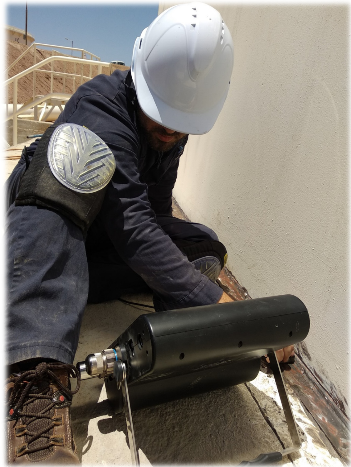
Inspection of annular rings for corrosion damages from the protrusion (outer chime)
