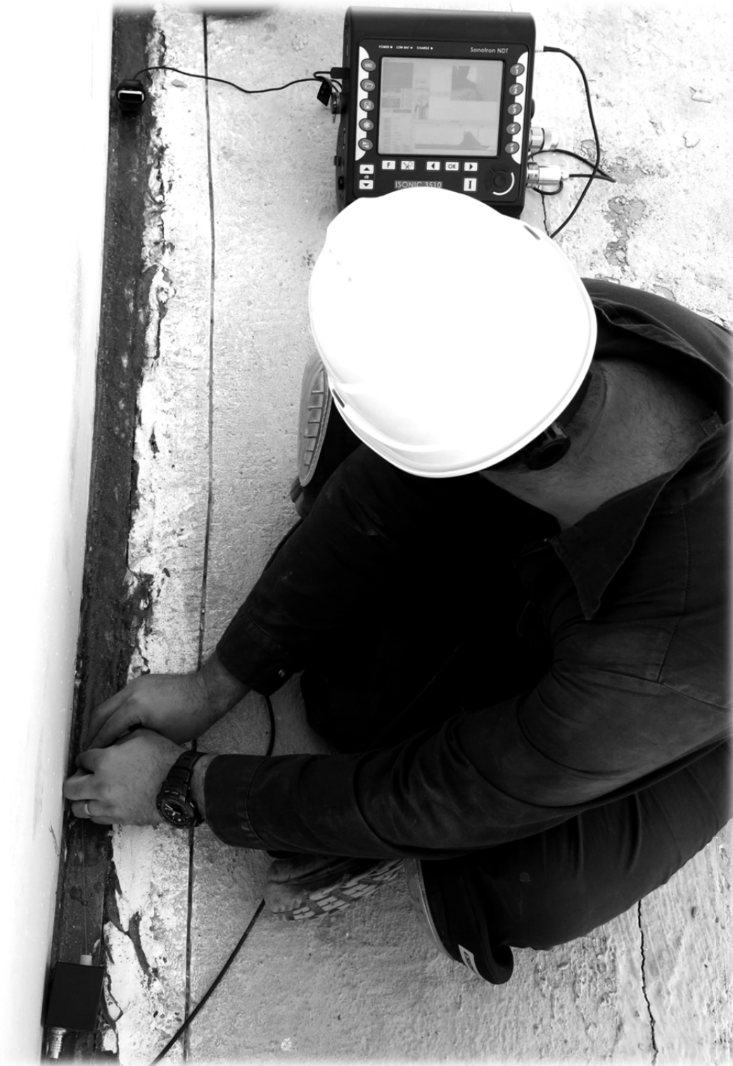
Inspection of annular rings for corrosion damages from the protrusion (outer chime)
