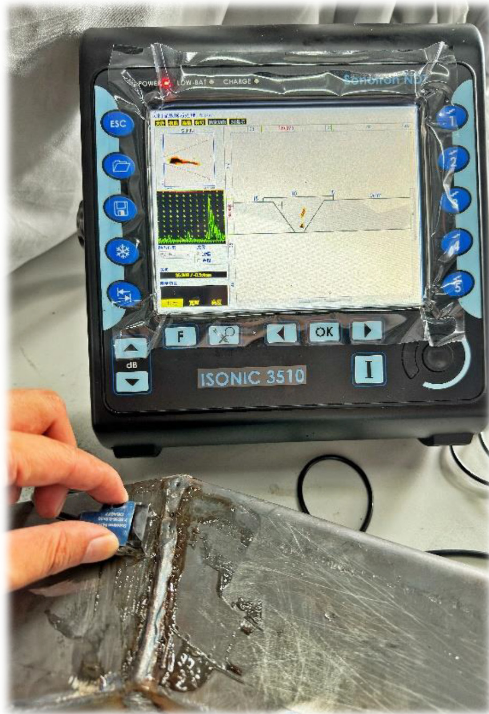
Structural butt weld and triple-wall butt weld between thin wall hollow rectangle profiles
