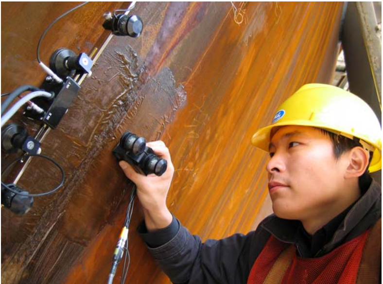
Airborne ultrasound based encoding of probe position and swiveling angle
