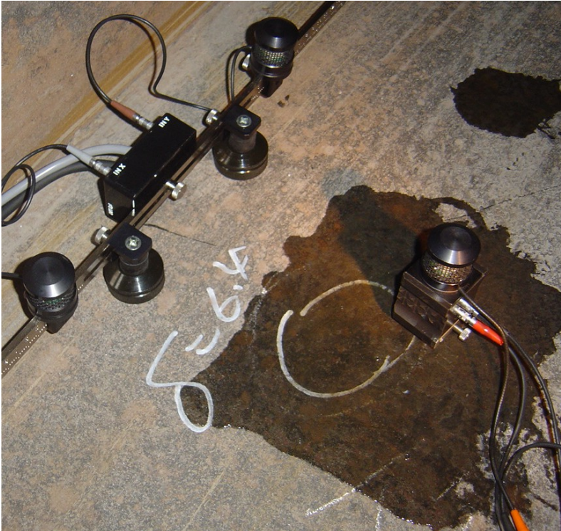
Airborne ultrasound based encoding of probe position only
